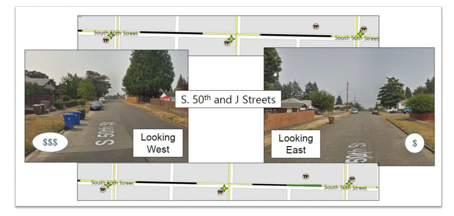
On the west side of J, there are no power poles next to the dark street segment. In order to add a light, a new wood pole and overhead line would need to be installed. On the east side of J, there is an existing TPU pole. Part of the dark segment can be lit up (shown in green) by attaching a new light to the existing pole.
